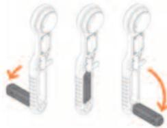
The handle revolves, allowing the operator to ergonomically and easily maintain control of the lever through its full 360° range of motion.
